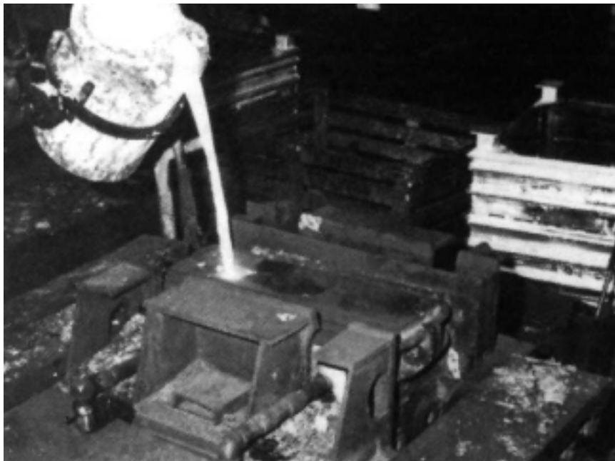
FIG. 13 — Permanent-Mold Casting for Fittings Production
