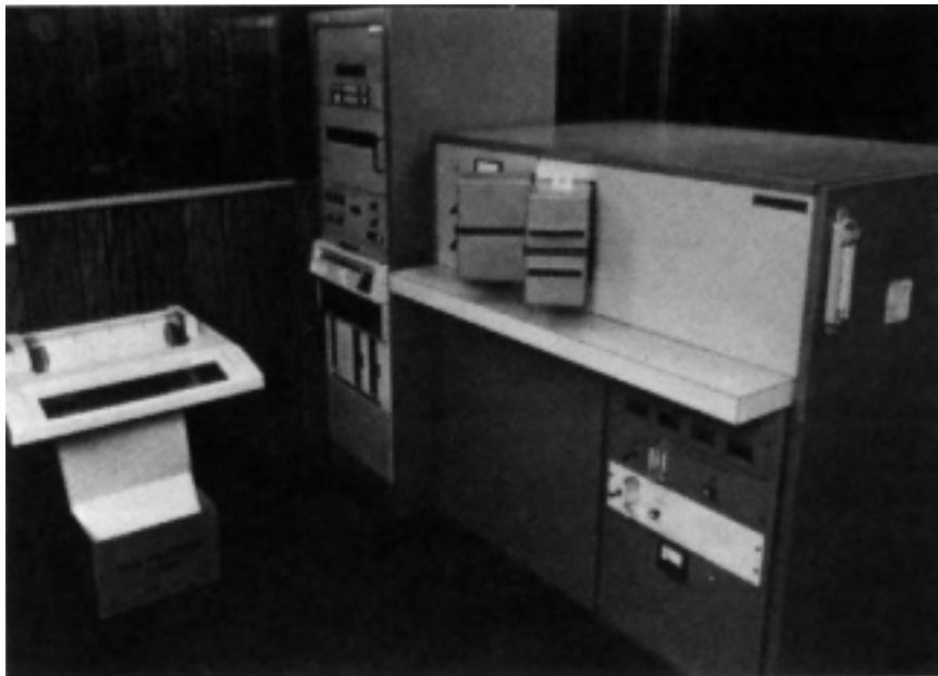
FIG. 24 —Optical Emission Spectrometer (OES) — Analysis of irons, production control samples and final product
