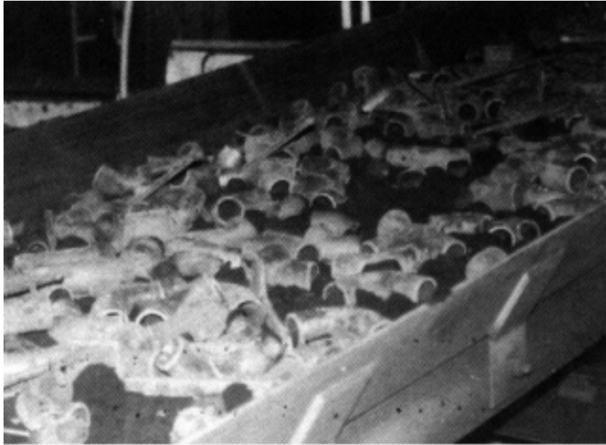
FIG. 17 — Castings Being Shaken Out of the Mold
