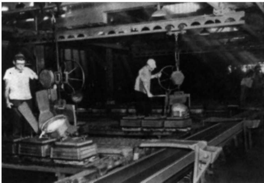
FIG. 12 — Pouring of Cast Iron Soil Pipe Fittings
