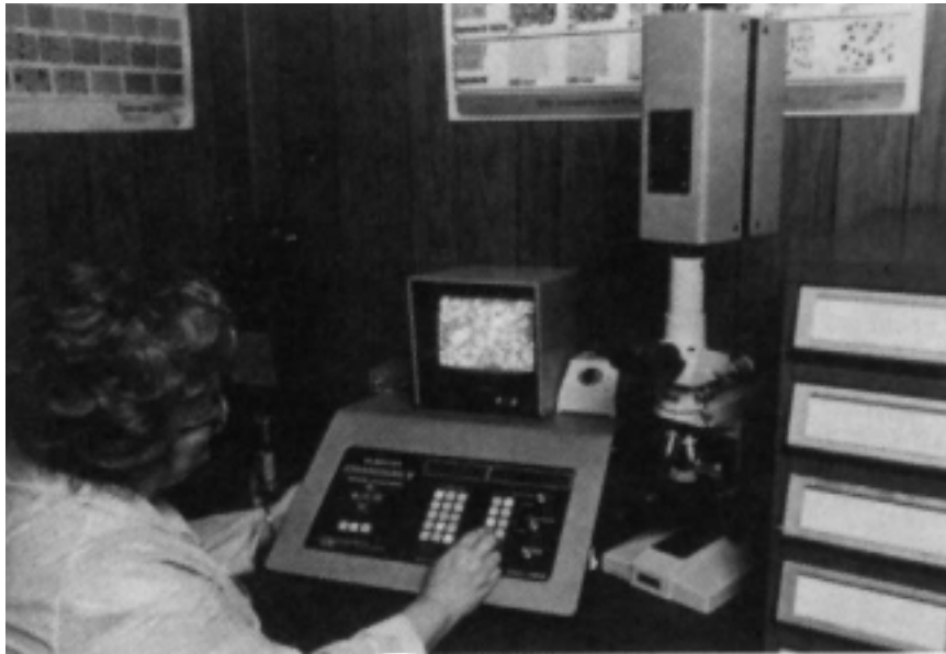
FIG. 23 — Image Analyzer — Defining the microstructure matrix of final product.
