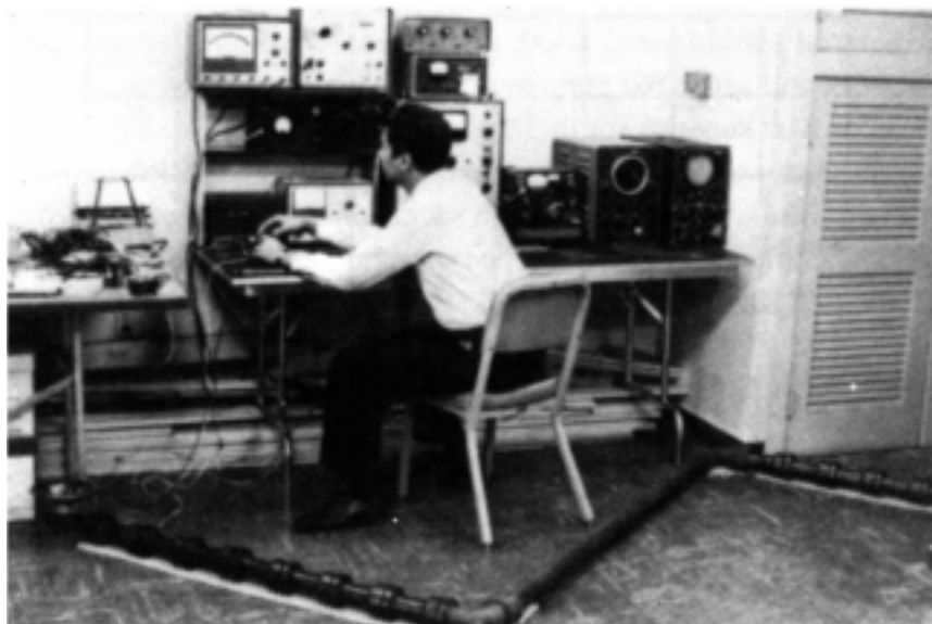
FIG. 5 — A "Z" Rig Being Tested for Acoustical Characteristics (Cast Iron with Neoprene Compression Gaskets)
