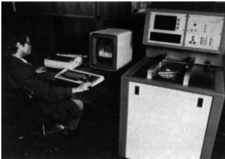
FIG. 22 — Energy Dispersive X-Ray Spectrometer — Analysis of iron, slag and raw materials.
