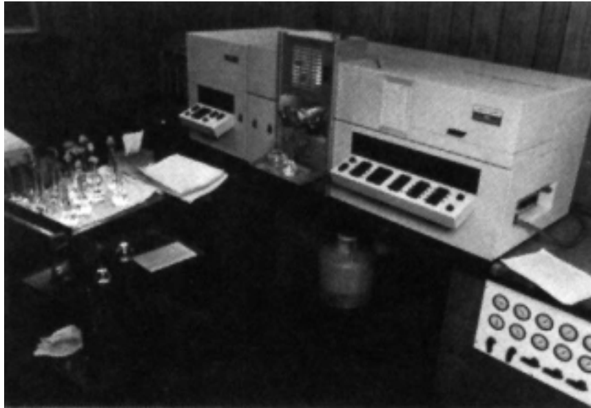
FIG. 21 — Atomic Absorption Spectrophotometer — Analysis of environmental samples, raw materials, control checks of optical emission and X-ray spectrometers.
