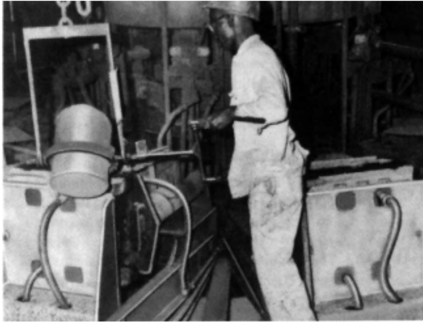
FIG. 14 — Rotating Wheel-Type Machine for Fittings Production
