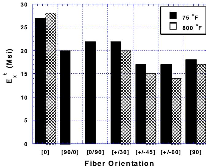
**FIGURE 3.8.2.1(h)** Average tensile modulus as a function of fiber orientation and temperature tested at strain rates of  $1 \cdot 10^{-3}$  and  $1 \cdot 10^{-4} \text{ s}^{-1}$ .
