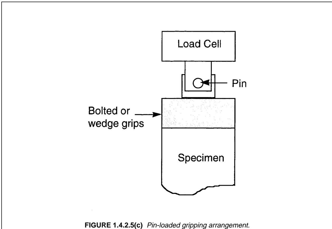
**FIGURE 1.4.2.5(c)** *Pin-loaded gripping arrangement.*
