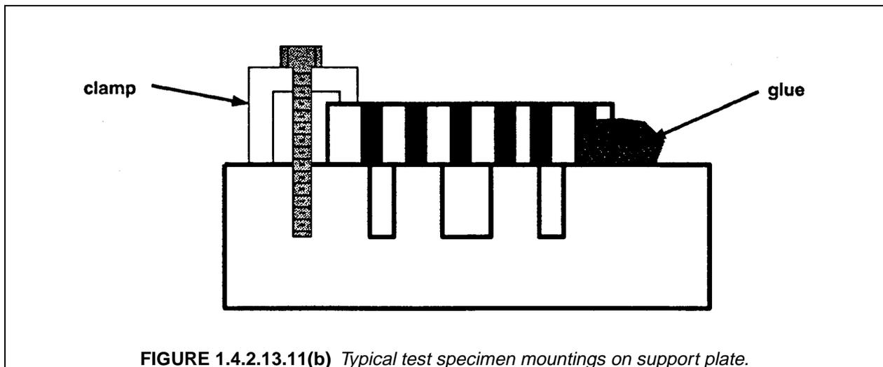
At this time, if the test specimen has more than one fiber that requires testing, a low magnification photograph of the specimen mounted on the support plate should be taken. This photograph will serve as a reference for locating the fibers of interest during and after testing.
