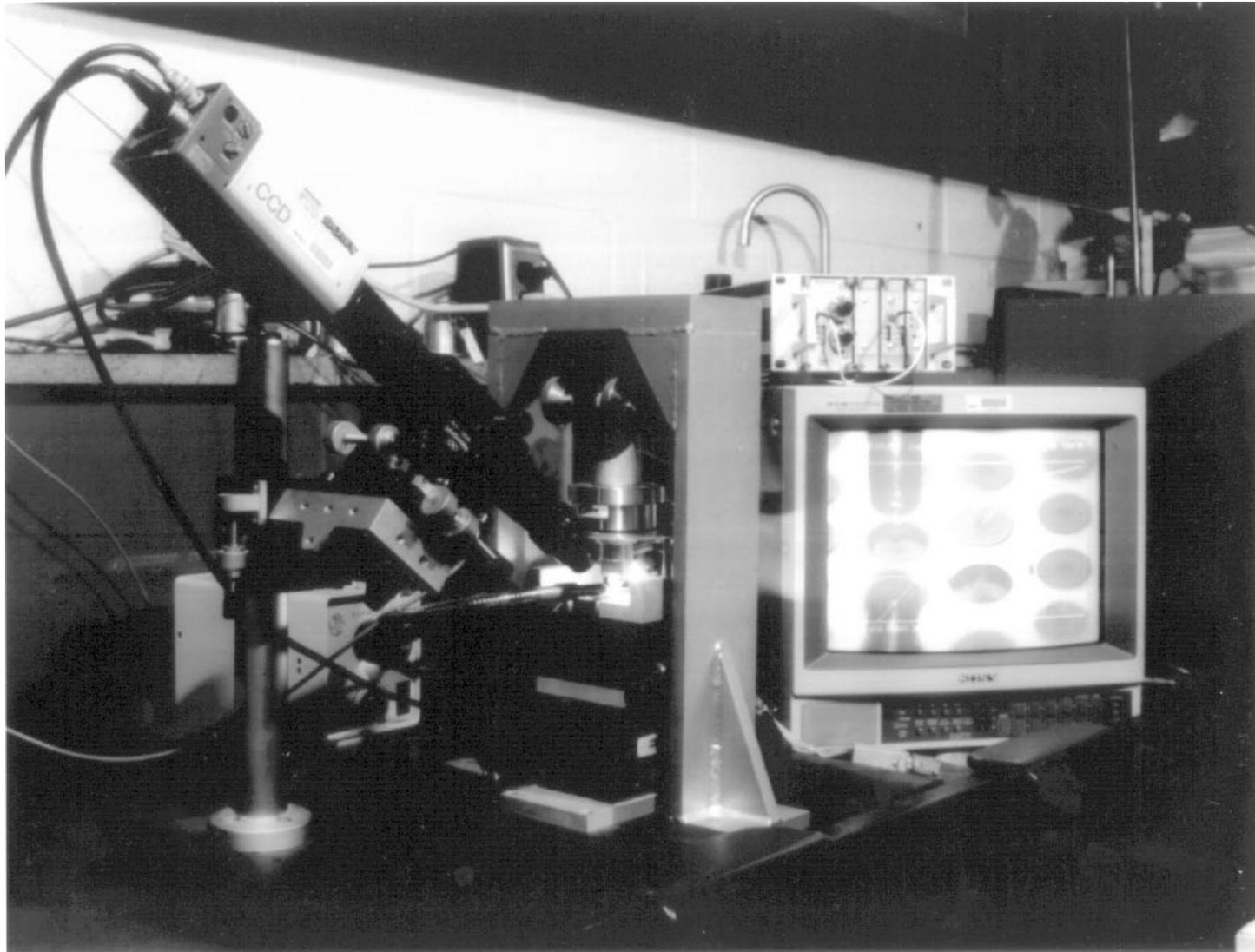
**FIGURE 1.4.2.13.5(b)** *Tabletop fiber pushout testing system used at NASA Lewis Research Center.*
