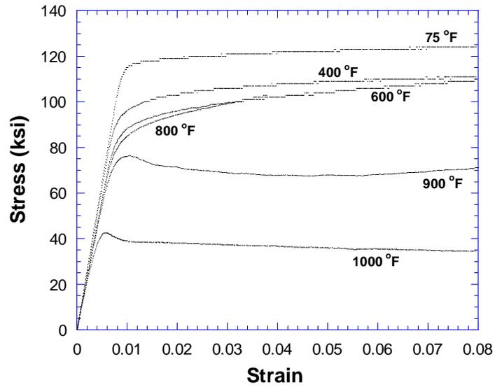
FIGURE 3.3.5.1(i) Tensile curves at a strain rate of  $10^{-4} \text{ s}^{-1}$  as a function of temperature.
