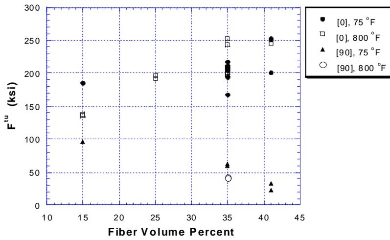
FIGURE 3.8.2.1(a) Ultimate tensile strength as a function of fiber volume and temperature.
