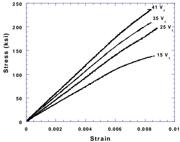
**FIGURE 3.8.2.1(f)** Typical tensile behavior of  $[0]_s$  laminae at  $800^\circ\text{F}$  ( $427^\circ\text{C}$ ) as a function of fiber volume percent ( $V_f$ ) at a strain rate of  $1 \cdot 10^{-3} \text{ s}^{-1}$ .
