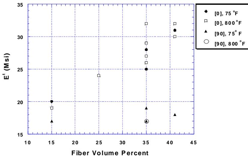
FIGURE 3.8.2.1(b) Tensile modulus as a function of fiber volume and temperature.
