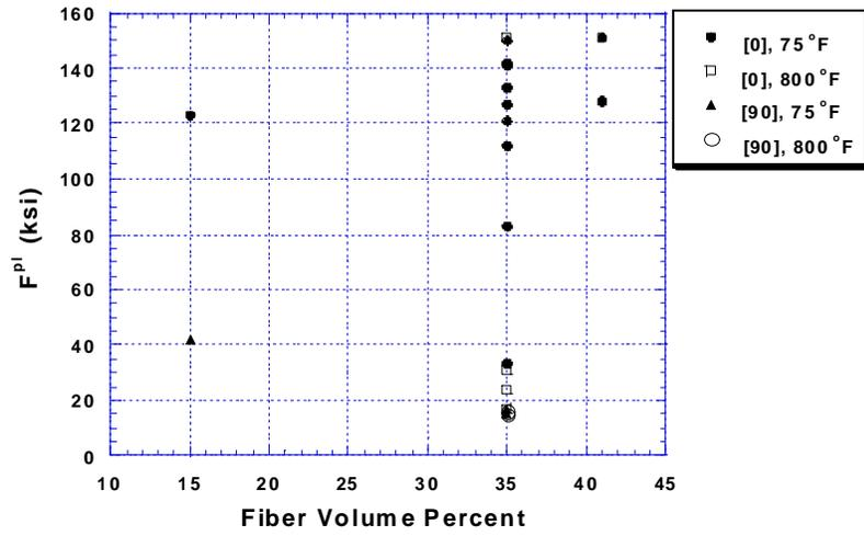
FIGURE 3.8.2.1(c) Proportional limit as a function of fiber volume and temperature.
