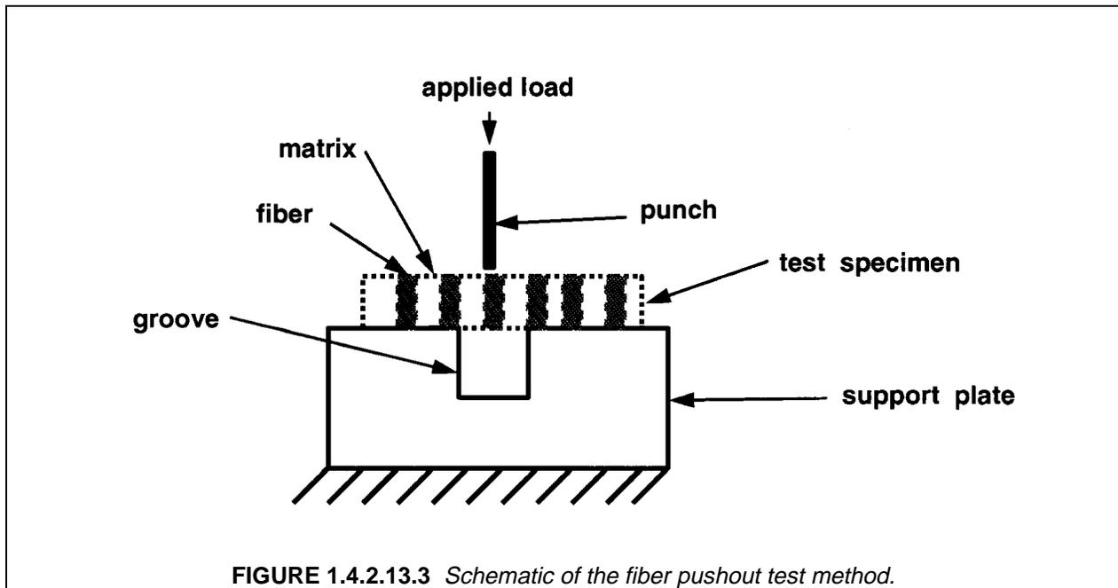
FIGURE 1.4.2.13.3 Schematic of the fiber pushout test method.
