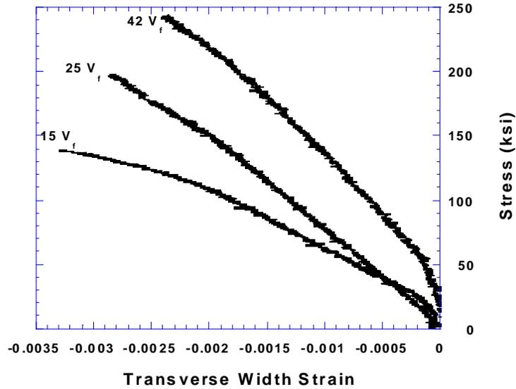
**FIGURE 3.8.2.1(g)** Typical tensile behavior of  $[0]_{\theta}$  laminae at  $800^{\circ}\text{F}$  ( $427^{\circ}\text{C}$ ) as a function of fiber volume percent ( $V_f$ ) at a strain rate of  $1 \cdot 10^{-3} \text{ s}^{-1}$ .
