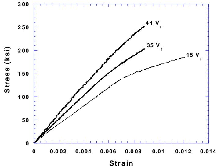
**FIGURE 3.8.2.1(e)** Typical tensile behavior of  $[0]_s$  laminae at  $75^\circ\text{F}$  ( $24^\circ\text{C}$ ) as a function of fiber volume percent ( $V_f$ ) at a strain rate of  $1 \cdot 10^{-4} \text{ s}^{-1}$ .
