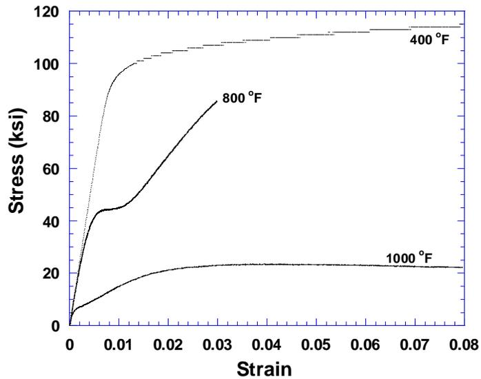
FIGURE 3.3.5.1(j) Tensile curves at a strain rate of  $10^{-6} \text{ s}^{-1}$  as a function of temperature.
