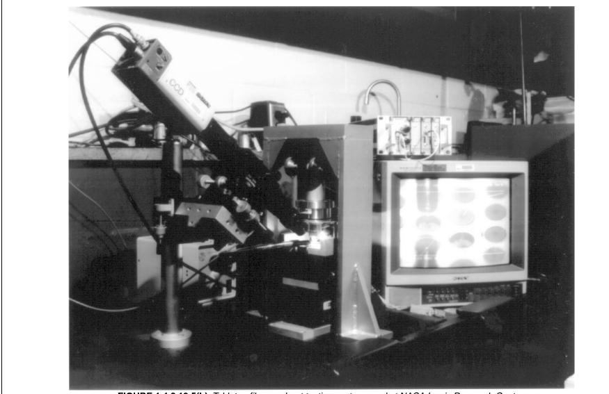
FIGURE 1.4.2.13.5(b) Tabletop fiber pushout testing system used at NASA Lewis Research Center.
