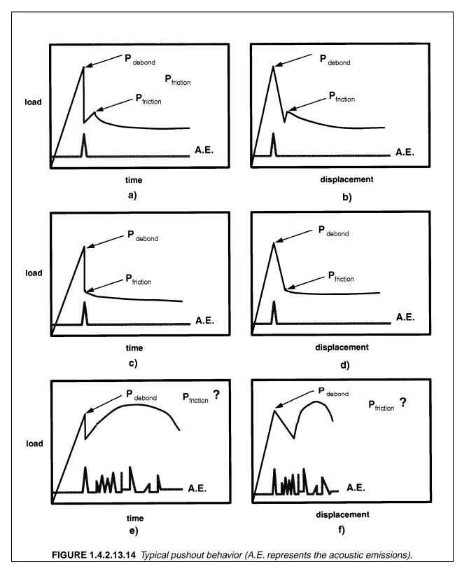
Occasionally, the load will again increase after the fiber has debonded, as shown in Figure 1.4.2.13.14, e and f. Pushout behavior such as this is more difficult to interpret, since following the debonding event the fiber does not slide freely. In such cases, extreme interface roughness or interfacial debris results in interlocking, which further resists fiber displacement. As a result the load increases and
