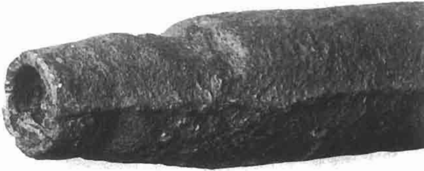
Fig. 1-4 End socket of a cast-iron waterpipe sealed with lead laid in 1457 (photo: Rheinstahl, Gelsenkirchen).
