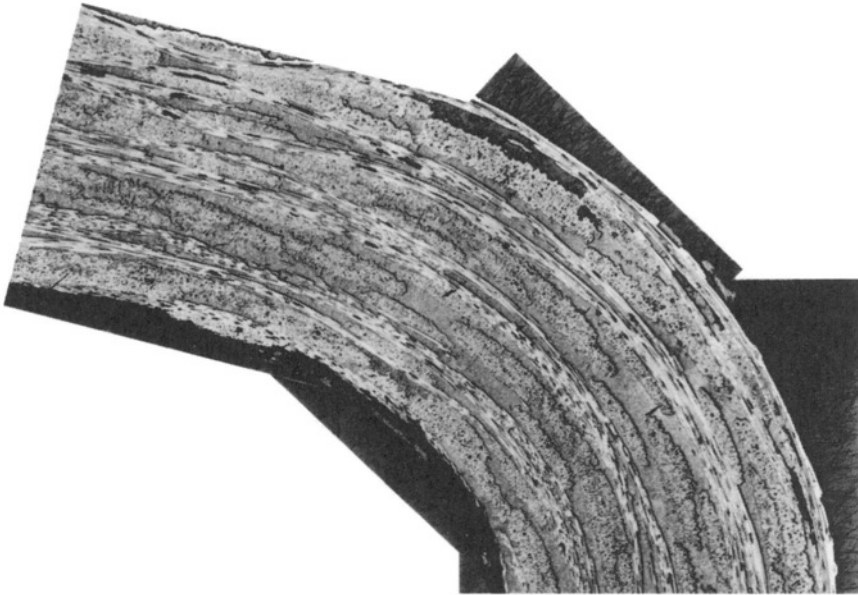
FIGURE 20. Microstructure of a curved section from a 2-D Nicalon™/Al 2 O 3 component.
