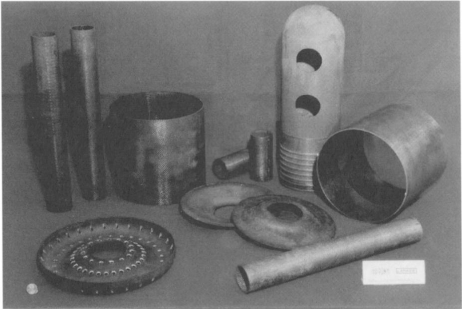
FIGURE 19. Nicalon™/Al 2 O 3 components fabricated using the directed metal oxidation process.
