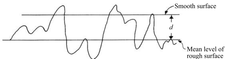
Figure 7.24 Approach of rough and smooth surfaces.
