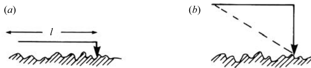
Figure 4.92 Effect of cranked stylus.
