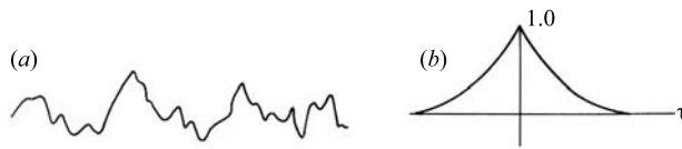
Figure 2.39 (a) Typical profile; (b) autocorrelation function.
