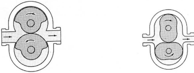
FIGURE 7 Typical single-lobe (left) and multiple-lobe (right) pumps
