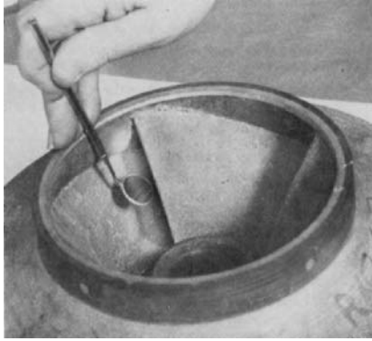
FIGURE 1 Examining the pressure side of the inlet vanes for suction recirculation damage
