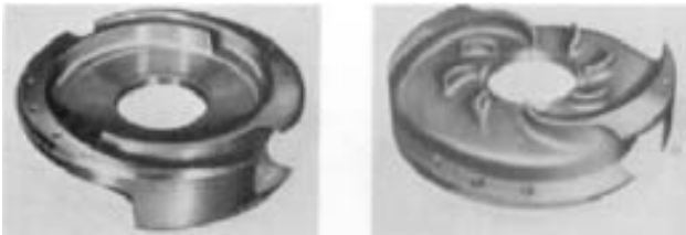
FIGURE 9 The double volute of a multistage pump, front view (left) and back view (right) (Flowserve Corporation)
