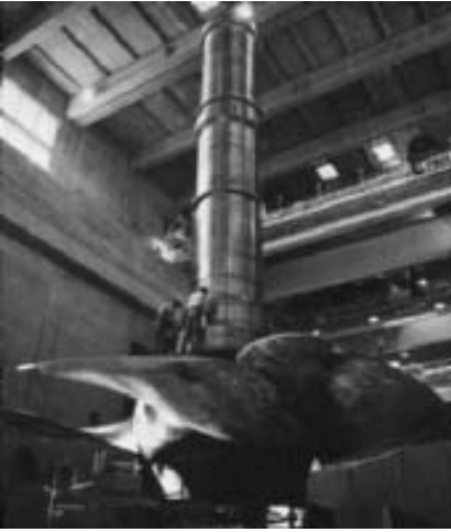
FIGURE 5 Adjustable-blade propeller runner. “Kaplan” turbines have adjustable blades coordinated with adjustable wicket gates (Voith Siemens Hydro)
