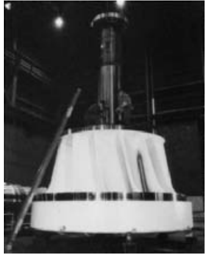
FIGURE 6 Francis runner has shorter buckets than a centrifugal pump impeller (Voith Siemens Hydro)
