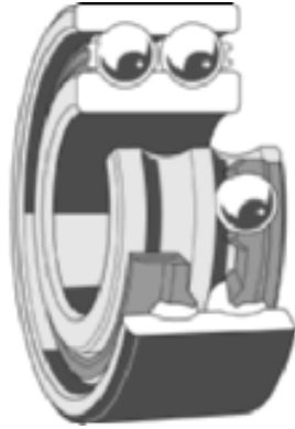
FIGURE 90 Double-row, angular contact bearing (SKF USA, Inc.)
