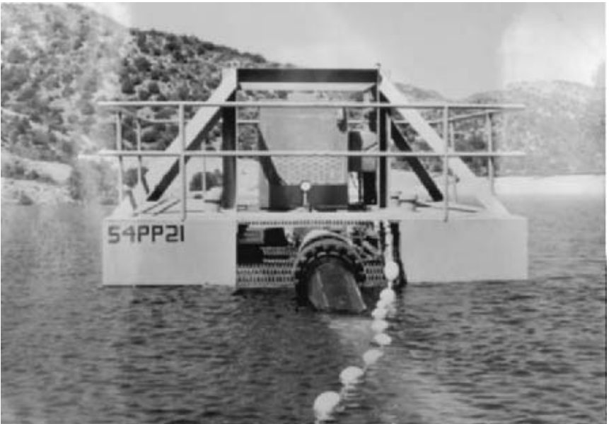
FIGURE 7 Unique design float-mounted pump (Hazleton Pumps, Inc.)
