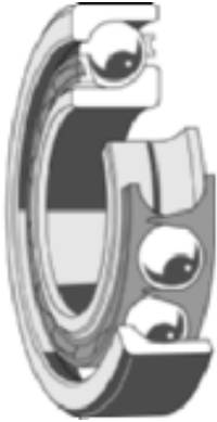
FIGURE 89 Single-row, angular contact bearing (SKF USA, Inc.)
