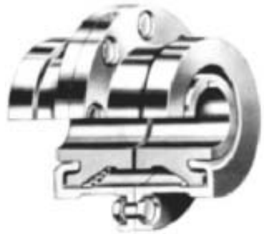
FIGURE 4 Gear-type mechanically flexible coupling (Kop-Flex)
