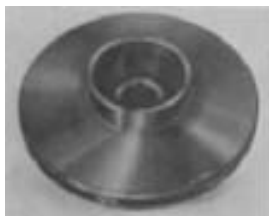
FIGURE 25 Straight-vane, radial, single-suction closed impeller (Flowsolve Corporation)
