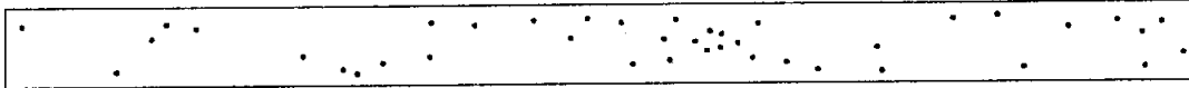
Typical Quantity and Size Permitted in 6 in. (152 mm) Length of Weld 1/8 in. (3.2 mm) to 1/4 in. (6 mm) Thickness
