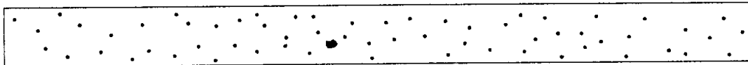
Typical Quantity and Size Permitted in 6 in. (152 mm) Length of Weld Over 1/4 in. (6 mm) to 1/2 in. (13 mm) Thickness
