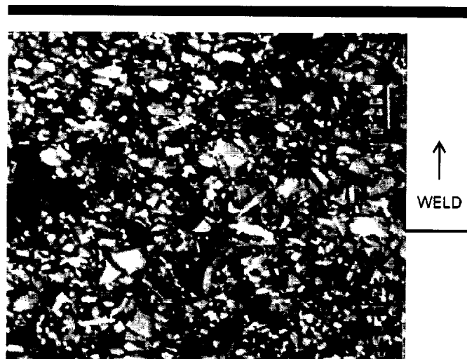
Figure 7.26—Unreacted SiC in Capacitor-Discharge Welded Joint (x800, unetched)
