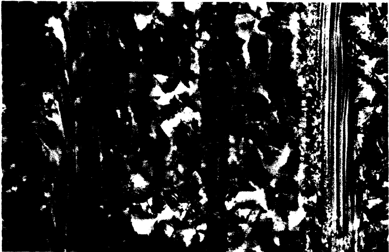
Figure 6.27—Polymer Morphology in Hot-Plate Welded Polypropylene
