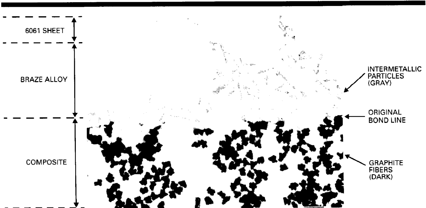
Figure 7.36—Brazed Interface Between 6061 Sheet and Al-7Zn/C with 718 as Braze Alloy (x500)
