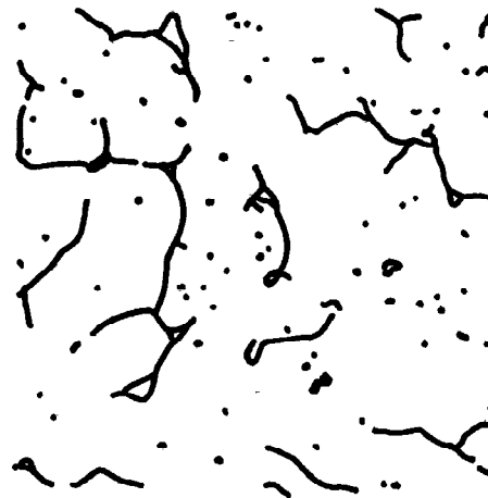
Fig. 2.5—Microstructure of E308 austenitic stainless steel weld metal with pools of delta ferrite
