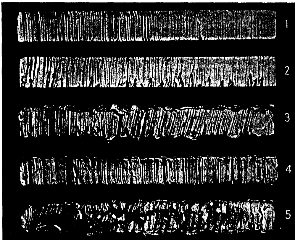
Figure 14.22—Typical Edge Conditions Resulting From Oxyfuel Gas Cutting Operations: (1) Good Cut in 1 in. (25 mm) Plate - the Edge is Square, and the Drag Lines are Essentially Vertical and Not Too Pronounced; (2) Preheat Flames Were Too Small for This Cut, and the Cutting Speed Was Too Slow, Causing Bad Gouging at the Bottom; (3) Preheating Flames Were Too Long, With the Result That the Top Surface Melted Over, the Cut Edge is Irregular, and There is an Excessive Amount of Adhering Slag; (4) Oxygen Pressure Was Too Low, With the Result That the Top Edge Melted Over Because of the Slow Cutting Speed; (5) Oxygen Pressure Was Too High and the Nozzle Size Too Small, With the Result That Control of the Cut Was Lost
