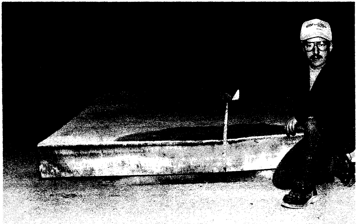
Figure 24.8—As-Explosion Clad Flat Plate Consisting of 13/16-Inch 304L Stainless Steel Clad on 8-Inch-Thick SA 516-70 Steel (DuPont photograph)
